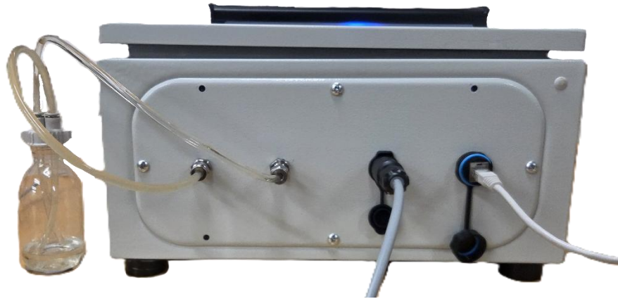
Figure 3A: BenchPro Installation with Sample Bottle (Front View)
